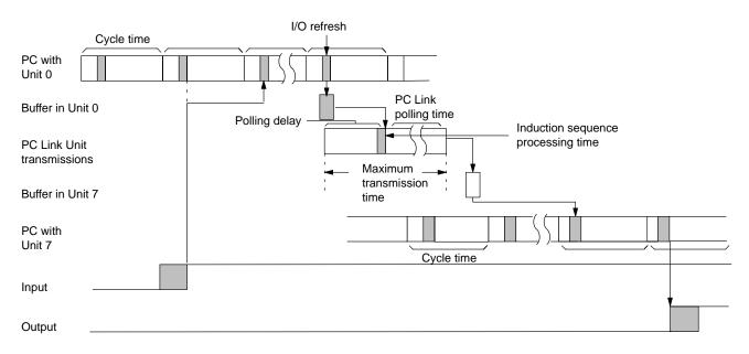
The equation for maximum I/O response time is thus as follows: Response time = Input ON delay + [Cycle time of PC of Unit 0 x (Number of LR transfer bits ÷ I/O refresh bits)] +  $\alpha$  + (PC Link polling time + Induction sequence processing time) + {Cycle time of PC of Unit 7 x [(Number of LR transfer bits ÷ I/O refresh bits) x 2 + 1]} +  $\beta$  + Output ON delay
